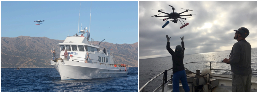
UAS operations from the M/V Magician, showing hand-deployments and catches of the APO-42 Octocopter.
