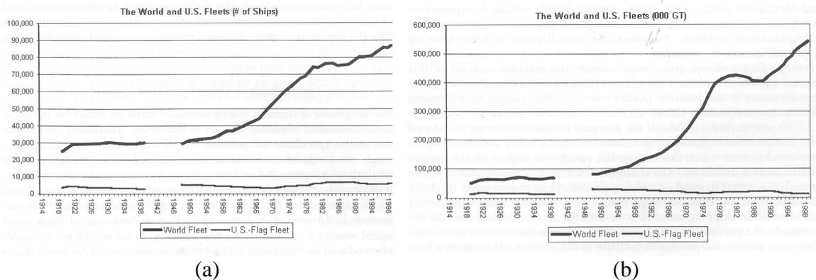
**Figure 1.** World and U.S. shipping fleet trends during the 20<sup>th</sup> century in terms of total numbers of vessels (a) and thousands of gross tons (b). (Source: National Research Council, 2003)
