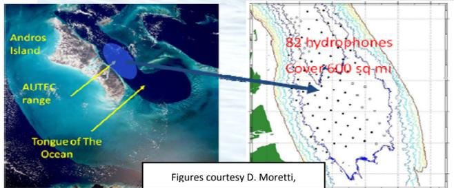
specialized underwater listening range (called the Atlantic Undersea Testing and Evaluation Center, or “AUTEK”) used by the U.S. Navy and its allies to train and test new equipment. Scientists and engineers
